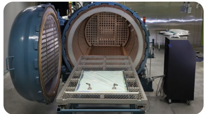
Uncured parts are put into special chambers called autoclaves. Autoclaves subject parts to pressure and heat to create finished composite parts.
