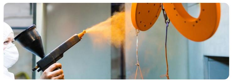
3M™ Polyester Tape 8992 is used to mask off areas from paint during the powder coating process.
