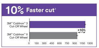
3. Results are based on an automated cutting of a 3mm thick 304 stainless steel sheet. Cut-off wheel geometry is  $125\text{mm} \times 1.6\text{mm} \times 22\text{mm}$  mounted on a 1.5 hp angle grinder with an applied force of 9 lbs. Cut speed is defined by time needed to cut 1 meter of stainless steel. The number of cuts is estimated by the amount of wheel that was used after cutting a distance of 1 meter. End of life is assumed to be 50% of initial wheel mass.
