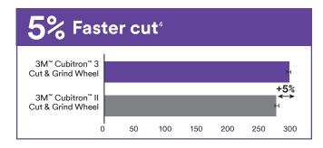
4. Results are based on an automated beveling of 1018 carbon steel bars. Cutting & grinding wheel geometry was 115mm outer diameter mounted on a servo motor with an applied force of 12 lbs. Cut speed is defined by metal removed after 10 minutes of testing. The total material removal is estimated based on the amount of wheel used for 10 minutes of testing life. End of life is assumed to be 50% of the initial wheel mass.
