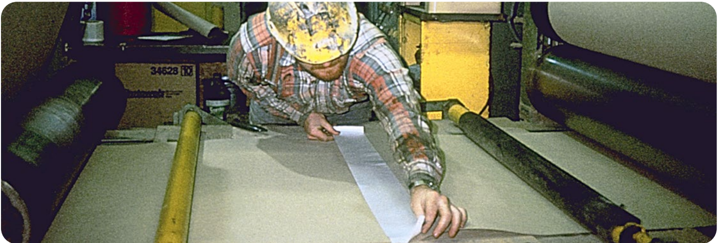
Worker applies 3M™ Thermosettable Glass Cloth Tape 365 to form a butt splice between heavy fabric rolls.
