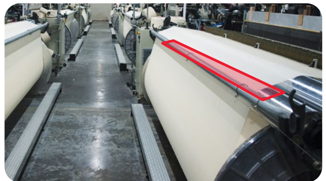
Outline indicating tape splice as it passes through a manufacturing process.
