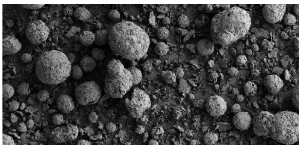
100 \mu m SEM micrograph: Grade CFA 250S
