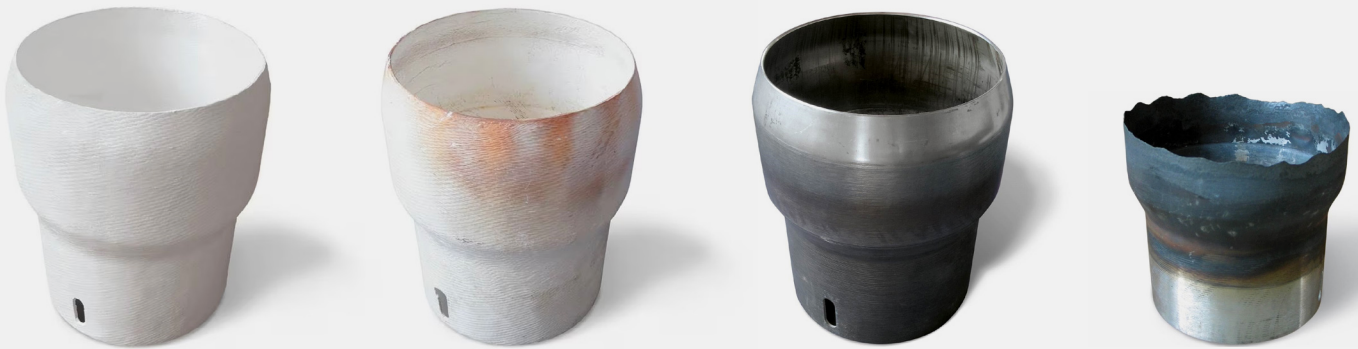
From left: Flame tubes made with Nextel ceramic sheets new and after 20,000 hours in use; metal flame tubes, type 1.4541, new and after 1,000 hours in use. Images courtesy of Walter Pritzkow.
