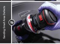
Sand the area with a 3M<sup>™</sup> Hookit<sup>™</sup> Purple Finishing Film Abrasive Disc 260L, grade P1500, 75 mm. Use disc with a soft interface pad. Remove all panel defects and match texture to adjacent OEM panels. Wipe panel clean
