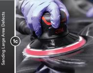
Sand the area with a 3M<sup>™</sup> Hookit<sup>™</sup> Purple Finishing Film Abrasive Disc 260L, grade P1500 - P2000, 150 mm. Use disc with a soft interface pad. Remove all panel defects and match texture to adjacent OEM panels. Wipe panel clean
