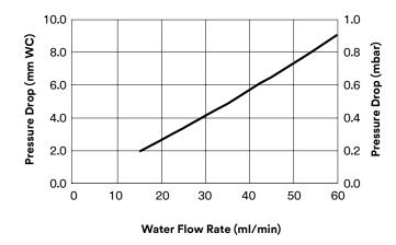
Test condition O₂ Removal: Vacuum mode with water at 35°C. Vacuum: 50 torr
