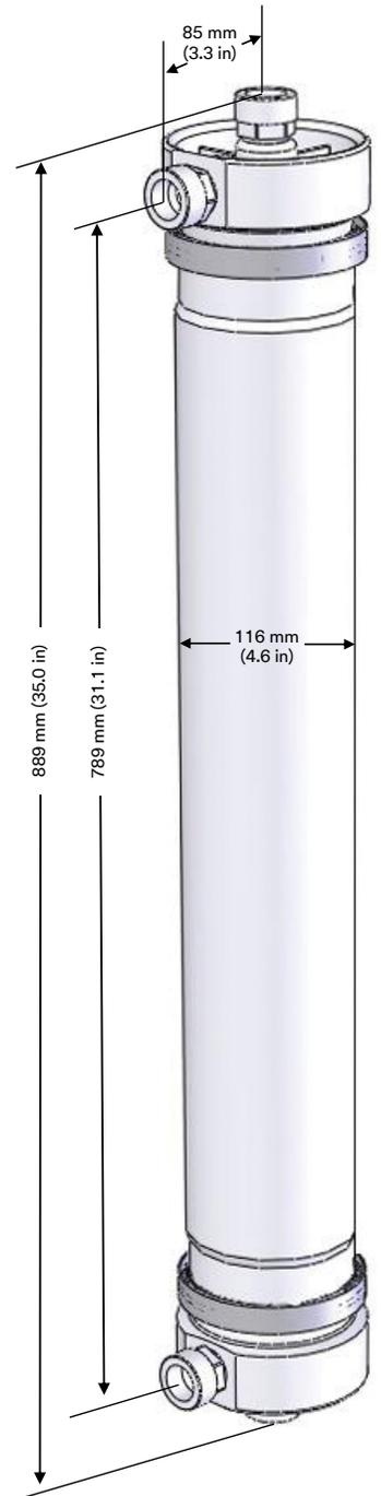
**All dimensions are nominal values for the polypropylene housing with NPT connections. See full housing drawing on 3M.ca/Liqui-Cel for additional details.**
