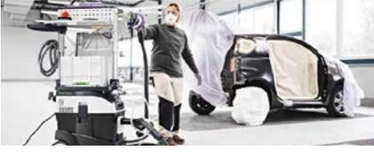
▶ Always use suitable dust extraction and select the correct tools for aluminum sanding: Festool Cleantec CTM 48 EC/B22 is certified under ATEX directive 94/9/EG for Zone 22 areas.
