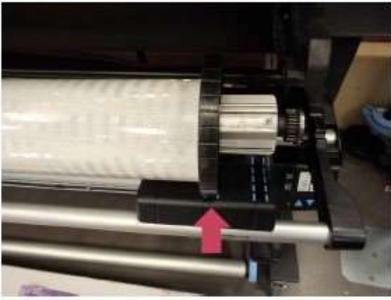
Figure 6. Proper traffic sheeting spindle loading location.
