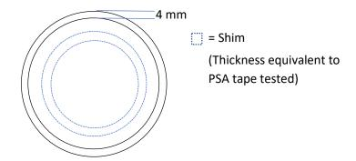
Due to the viscoelastic nature of PSA tapes, the applied pressure across the edge of simulated devices would be decreased due to the compression of the PSA tape. To account for this, it is necessary that samples are tested to the same pressures, with and without shims (at the same thickness as the PSA tape used), to maintain or compress the bond line, respectively. The simulated devices will be considered as passing the test when no visible liquid has entered the internal chamber of the device.
