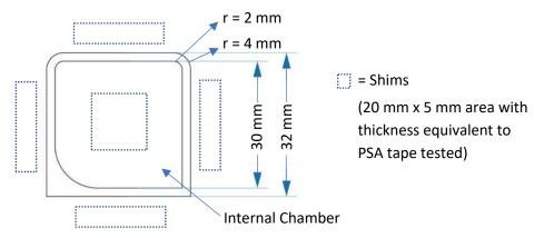
The test configuration for the 3M™ VHB™ Extrudable Tape is shown below in the black consistent lines while the shim is shown in the dashed line.
