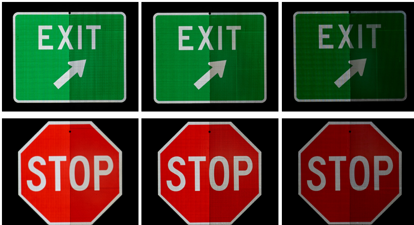
Signs fabricated with sheeting at a 90-degree orientation and photographed in a controlled lab setting.
