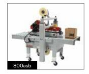
Seals up to 28 cs/min Max carton weight 38 kgs Side belt drives
