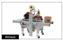
3M-Matic™ Case Sealer 800asb is an adjustable side belt drive case sealer designed for smaller, shelf ready cartons. Seals up to 28 cases per minute, using tape width of 36mm.
