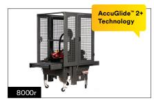
3M-Matic™ Case Sealer 8000r is a semiautomatic random case sealer automatically adjusts for case height and width. Top and bottom seal at rates up to 20 cases per minute, using tape widths from 36mm to 48mm wide.
