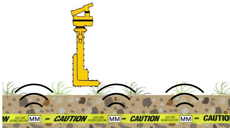
Figure 5: Cross-section signal pattern above path markers. Path markers are shown as “MM” on the EMS caution tape.
