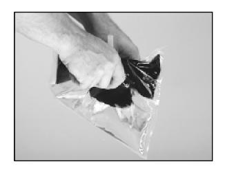
5.4 Separate barrier next to bag nozzle by positioning thumbs the same way as before. Allow compound to flow into the injection nozzle.
