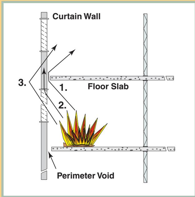
**Figure 1** – In unprotected construction, a curtain wall fire can propagate through the safing gap (1); through the window head transom and curtain wall cavity (2); and through broken windows or melted aluminum spandrel panels in the curtain wall above (3).
