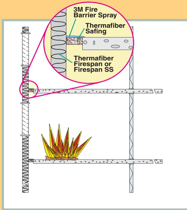
**Figure 2** – Effective curtain wall and perimeter void firestopping measures combine high quality Thermafiber insulation and 3M Fire Barrier Spray to protect both exterior curtain walls and the floor-to-wall gap.
