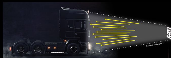
DG 3 Sign: More light reflected from sign; more reaching the driver's eye.
