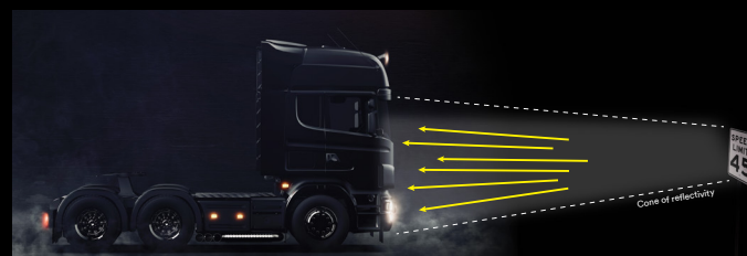
High Intensity Prismatic: Less light reflected from sign; most striking truck below the driver's eye.
