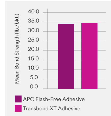
Figure 4: Bond Strength of APC Flash-Free vs. Transbond XT adhesive
