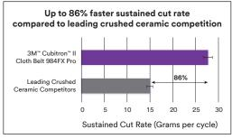
Results based on an automated, 10-minute grinding test on 304 stainless steel using 36" long belts. Error bars = 95% confidence interval. Cut rate: the total material removed in grams after 10 cycles minus total material removed in grams after 3 cycles divided by seven cycles. The unit is grams/cycles.
