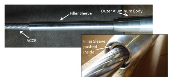
Press the large outer aluminum sleeve with the 100-ton (90.8 metric tons) press.
