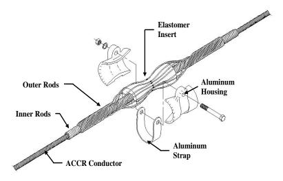
Helical-Rod Suspension Assembly from PLP.
