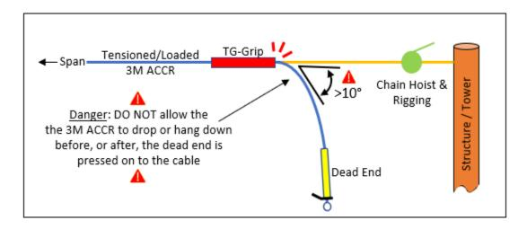
The compression dead end can now be connected to the insulator string and appropriate jumper connectors can then be installed. Brushing of the terminal pads of the dead end and jumper terminal with a wire brush is required. The use of AFL's Alnox® Electrical Joint Compound (EJC) or any other EJC approved by 3M for this application is required between the terminal pad and the dead-end pad for a good electrical connection.
