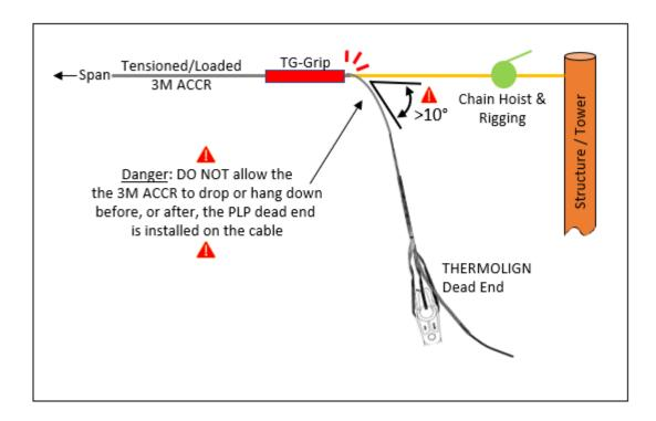
The chain hoist can now be removed along with the preformed conductor grip. These assemblies allow the conductor to pass through the dead end and create a "tail". This tail of the conductor will not be under any tension, can be cut to any length and used as a connector or jumper to the existing line. The pictures below show multiple ways to connect the jumper tail.
