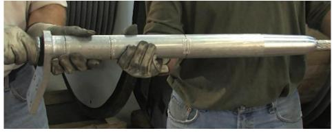
On some 3M ACCR sizes, the dead-end assembly also contains an aluminum filler sleeve that must be fitted inside of the larger outer aluminum body. This filler sleeve must be pushed into the outer aluminum body, so it is recessed inside of it.
