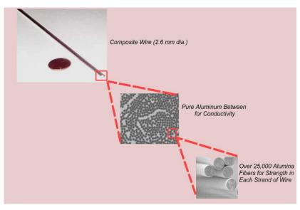
The composite wire provides high strength and conductivity at low weight.
