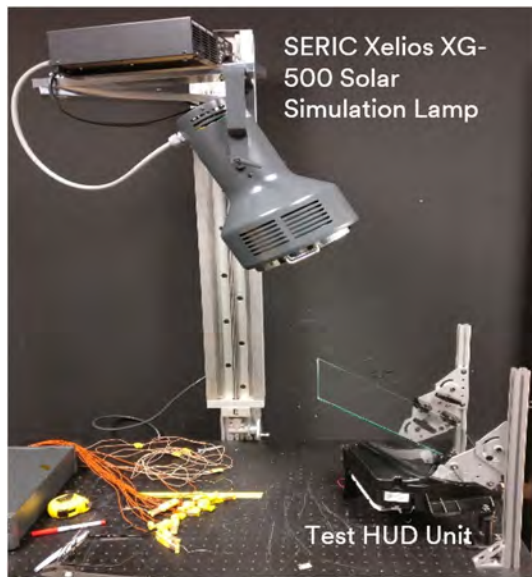
FIGURE 9 Experimental thermal measurement set-up to examine liquid crystal display (LCD) temperature reduction. HUD, head-up display
