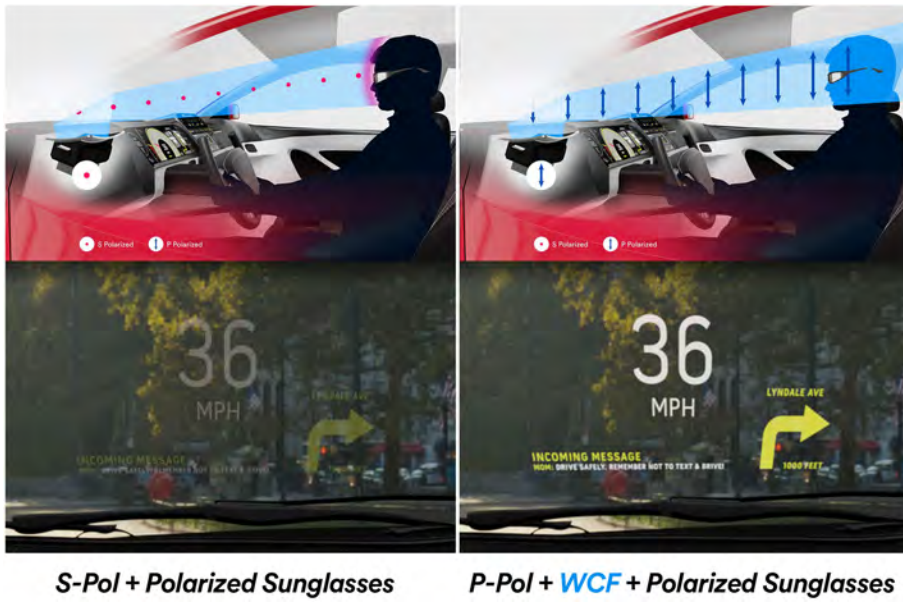
FIGURE 2 When a picture generating unit (PGU) projecting P-pol light is configured with a windshield combiner film (WCF) windshield, images are bright when seen through polarized sunglasses
