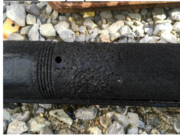
Picture 4: Black precipitation inside connection PP05
