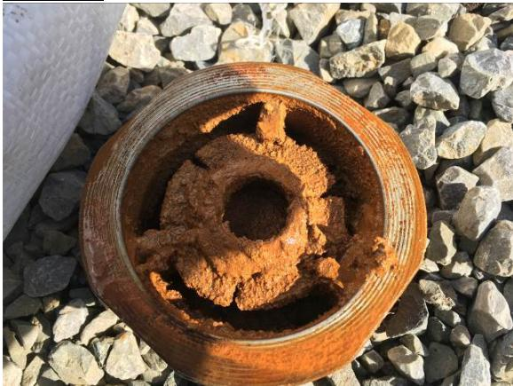
Picture 7: Dismanteled piping container
