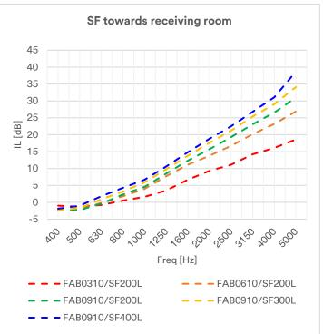
Note: 0.8 mm, 7.69g/cm3 steel panel was facing the noise source room and used in the insertion loss calculation
