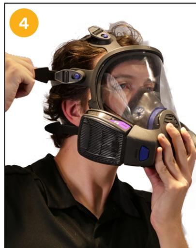
4. Tighten the two middle straps, then the two top straps. Make sure the back of the harness is centered on the back of the head and that the straps and tabs lay flat against your head.
