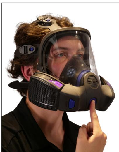
Lightly press the seal check button until you feel resistance. Hold the button in this position and exhale (blow out). If facepiece bulges slightly with no leaks detected between your face and the facepiece, a proper seal has been obtained.
