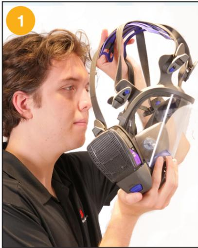
1. Fully loosen all six head straps. Hold the front of the facepiece with one hand and the straps/comfort cradle away from the facepiece with the other hand, creating an opening for the head.
