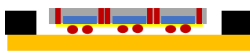
Fig. 1(b), the wafer form package bonds to the tape after frame attach
