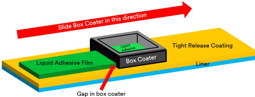
Figure 2 BYK Box Coater usage illustration
