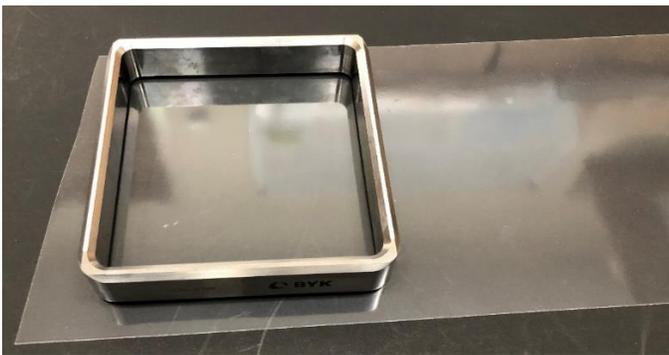
1. When using a box coater, double the thickness of your desired output to get the correct gap e.g., 50  $\mu\text{m}$  (2 mil) film thickness would need a 100  $\mu\text{m}$  (4-mil) gap.
