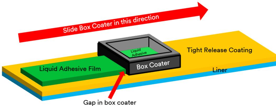
Figure 2 BYK Box Coater usage illustration
