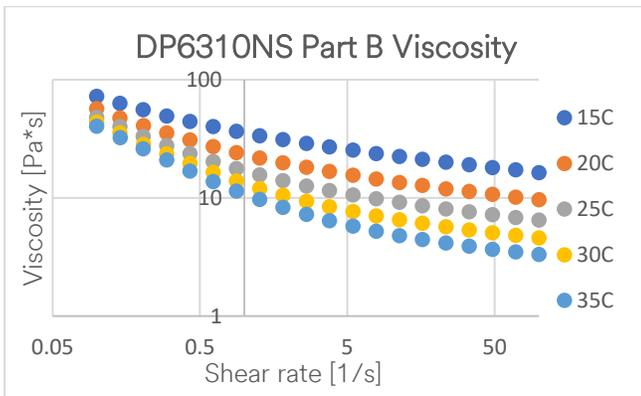
\*Note: Viscosity measurements done by cone and plate
