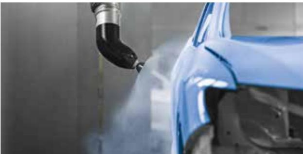
Clearcoat is sprayed on top of a colored basecoat and is a glossy and transparent coating that forms the final interface with the environment.
