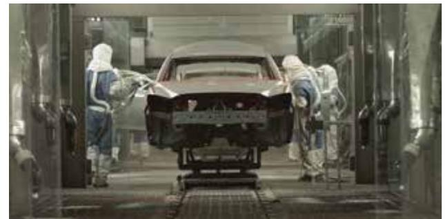
Basecoat contains the visual properties of color and effects and is usually the coat referred to as "paint."
