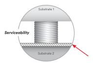
Single sided solution, allowing parts to be readily disassembled after cure for serviceability
