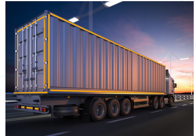
Effective conspicuity markings to keep vehicles visible
