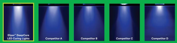
More homogeneous energy distribution throughout the restoration. Images comparing the light penetration of various light curing devices show that the Elipar DeepCure LED curing lights produce a more collimated and uniform beam profile – even in deeper areas.<sup>3</sup>
