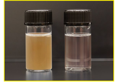
Before and after using 3M™ Harvest RC Chromatographic Clarifier: turbidity reduction in a single stage
