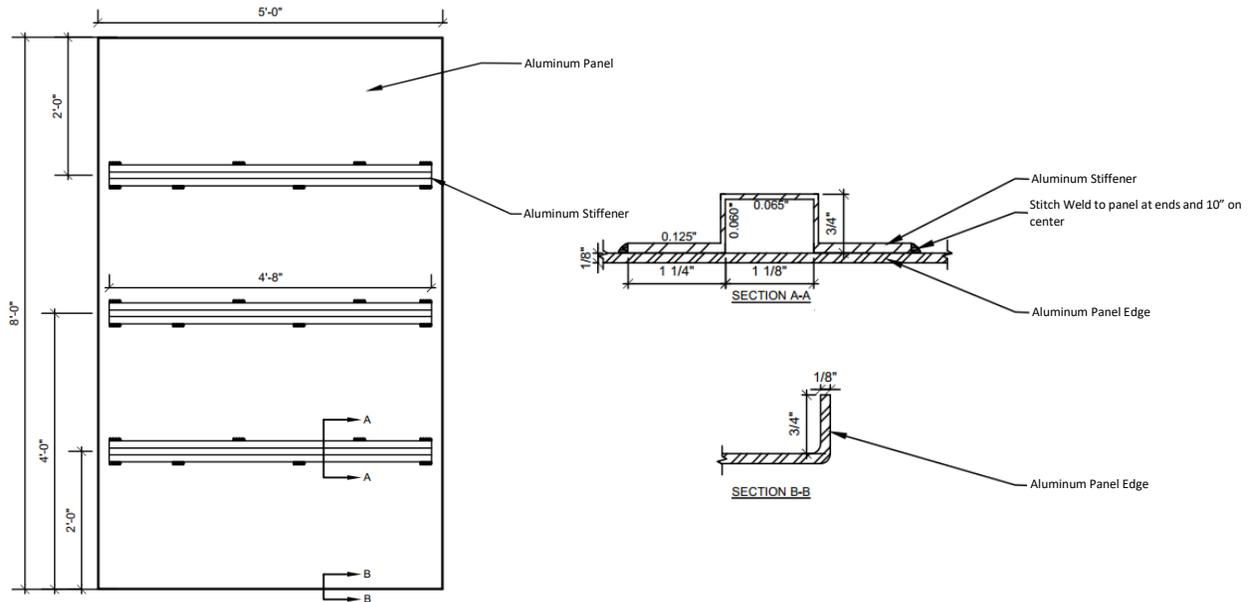
*Figures 6-8: Welded Panel Dimensions and Stiffener Attachment Method*
