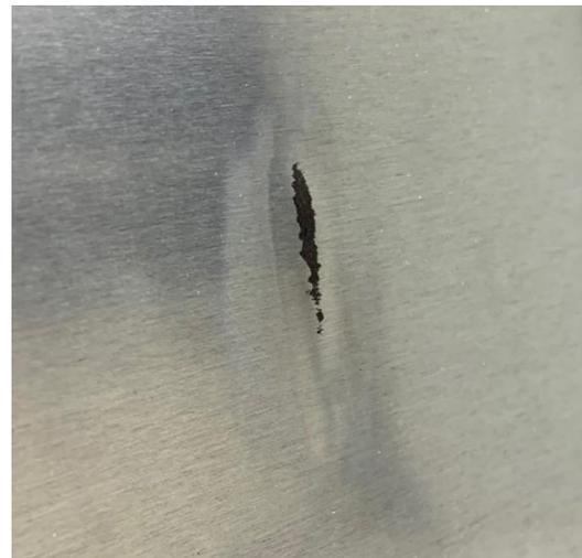
*Figure 10: Visible Weld Mark*
