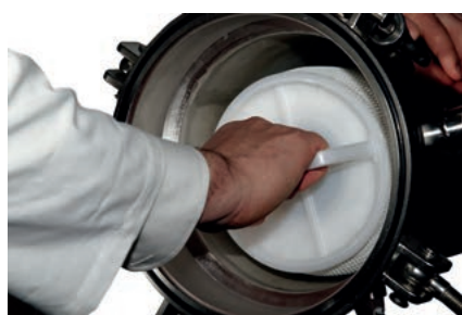
'Twist-to-lock' cartridge seating mechanism
