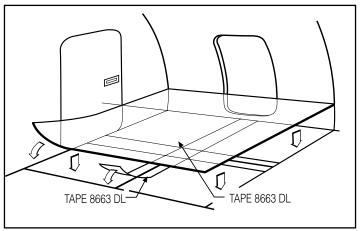
Transparent color allows visual inspection through material without removal.
