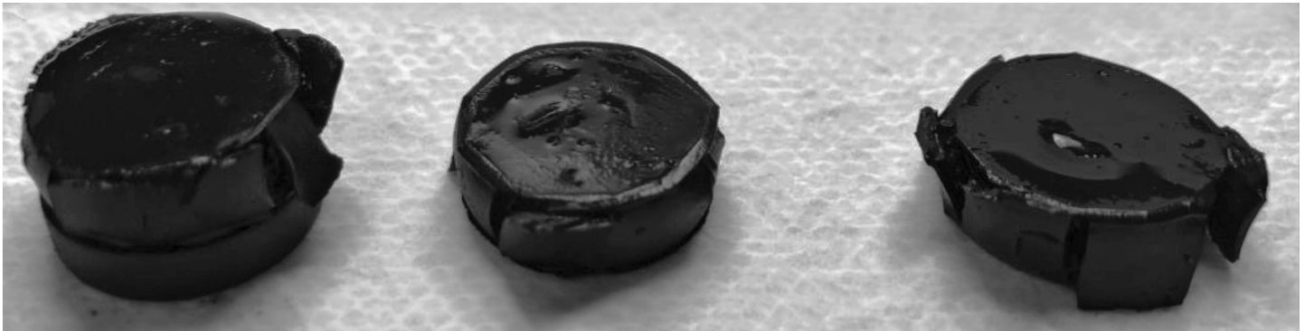
Figure 1: HNBR CSR buttons after 3024 hours exposure in Prestone® Coolant
