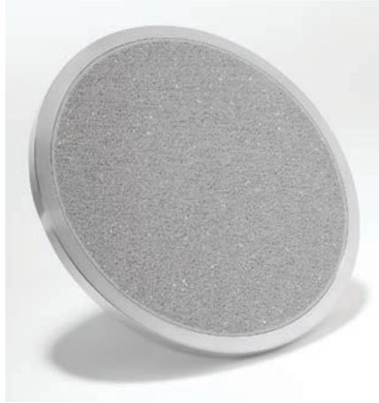
3M™ Diamond Pad Conditioners use 3M's exclusive sintered abrasive technology to provide a powerful chemical and mechanical bond between diamonds and substrate, helping keep diamonds intact and in place for consistent long-term conditioning performance.
