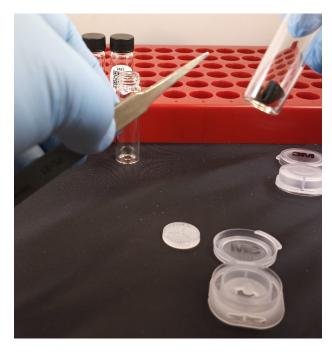
Add ca. 50 mg sodium carbonate to the vial to neutralize excess HBr present on the wafer. (The sodium carbonate will not dissolve.) Pipet 2.0 ml of Internal Standard Solution and cap the vial with inert, gas-tight closure. Agitate the vial continuously for one hour using an orbital shaker or equivalent. Reserve for gas chromatographic analysis.
