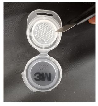
Using clean forceps, transfer the carbon wafer into a 7 ml glass vial (or similar) with inert gas tight closure cap.
