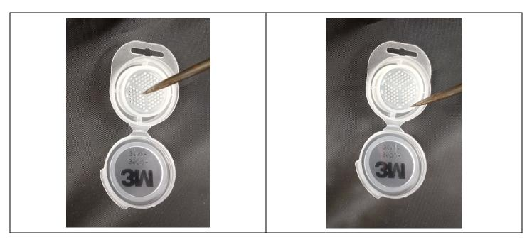
If you do not have a pick, use a small sharp blade to make 2 incisions within 25 degrees for each other. Then pry the sampling grid out.
