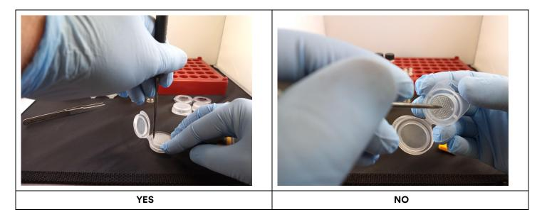
Using a lab pick (e.g., McMaster-Carr 3842A42) as a tool, remove the plastic Sampling Grid from the clear plastic Sampler Body exposing the yellow glass fiber wafer beneath. Place the tip of the pick either at the side or the middle. Push down hard and pry out the sampling grid.
