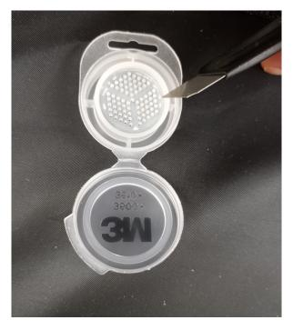
Using clean forceps, place the glass fiber wafer in an inert filtration vial (e.g., Syringeless Filter Vial, 0.45?m PVDF, Whatman Item No UN513VAQU).
