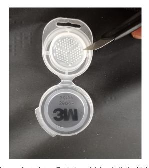
Using clean forceps, transfer the carbon wafer to into a 7 ml glass vial. (or similar) with inert gas tight closure cap.
