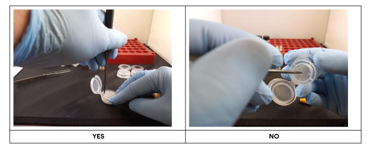
Using a lab pick (typ. McMaster-Carr 3842A42) as a tool, remove the plastic Sampling Grid from the clear plastic Sampler Body exposing the carbon wafer beneath. Place the tip of the pick either at the side or the middle. Push down hard and pry out the sampling grid.
