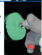
1. Compound the abraded surface with 3M™ Perfect-It™ Fast Cut Plus Extreme and  $3M^{\mathsf{TM}}$  Perfect- $\mathsf{It}^{\mathsf{TM}}$  Low Linting Wool Compounding Pad or 3M™ Perfect-It™ Green Foam Compounding Pad. Use a Rotary Polishing machine at a speed of 1400 - 1800 rpm's.
