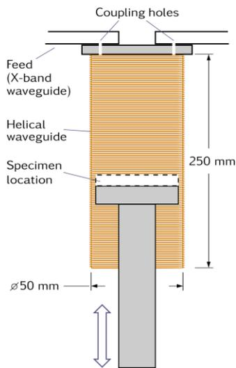
Figure 2: Helical cavity (used at NPL)
