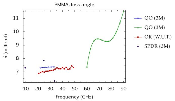
Figure 8: PMMA measurements
