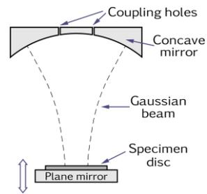
Figure 4: Plano-concave open resonator (used at NPL)
