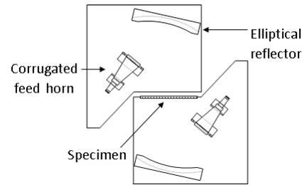
Figure 5: Free-space transmission system (used at 3M)
