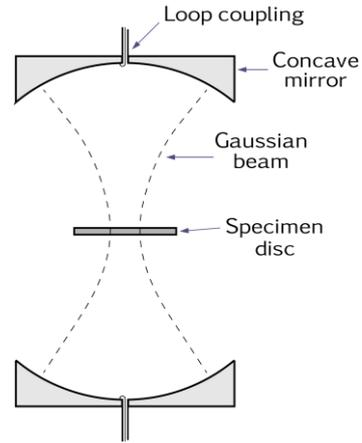
Figure 3: Bi-concave open resonator (used at W.U.T.)
