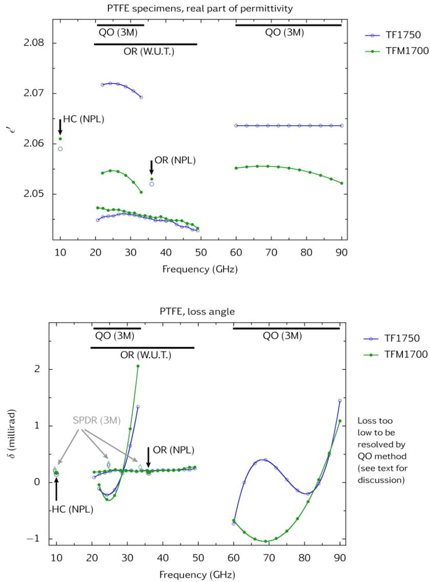
Figure 6: Measured permittivity and loss angle for two grades of PTFE. Bracketed values are uncertainties at coverage factor  $k=2$  (equivalent to approx. 95% confidence level).
