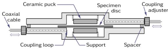
Figure 1: Split-Post Dielectric Resonator (used at 3M)
