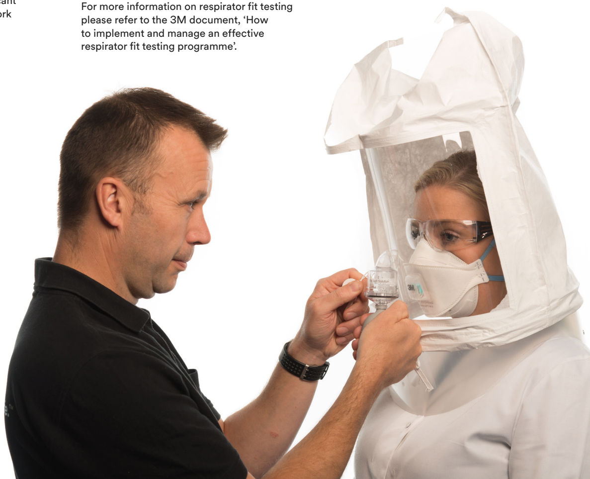
Figure 3. 3M™ Qualitative Fit Test Apparatus Kit and Bitrex® Fit Test kit being used to conduct a Qualitative Fit Test (QLFT) upon a subject wearing a filtering facepiece respirator
