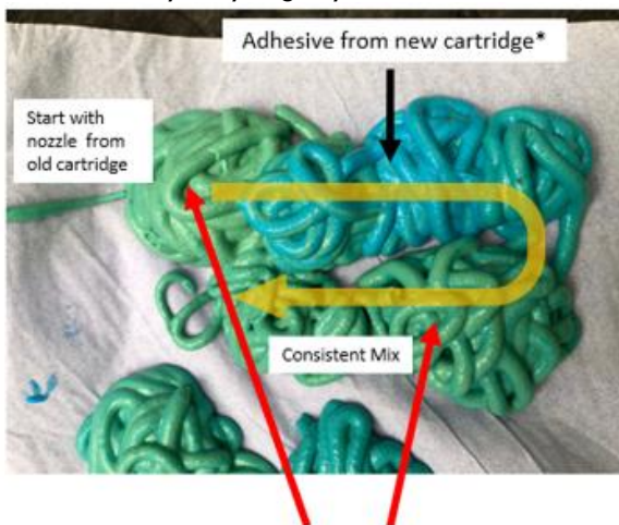
Homogeneous green color indicating correct mix ratio and good mix
