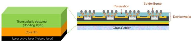
**Figure 2,** 3M laser releasable temporary bonding de-bonding film (multi-layered product) for supporting RDL-last process
