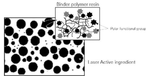
**Figure 7**, Design concept of 3M laser releasable temporary bonding film (single layered product)
