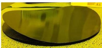
**Figure 1.** Delamination between a carrier and a device due to severe device warpage during high temperature processing. If the gripping
