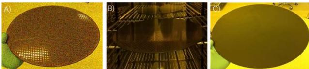
**Figure 3,** Passivation curing simulation test (230 °C X 2hrs X 2 Times) for actual bonding wafer with 3M product, A) Bonded device with carrier by using 3M product, B) Maintaining grip force of 3M product for glass carrier during passivation layer curing process, C) Mold wafer after carrier de-bonding & adhesive peeling; Device wafer without warpage & adhesive residue.
