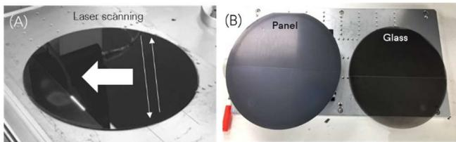
**Figure 9,** Laser de-bonding processing, (A) Laser scanning, (B) Demounted device wafer from a carrier
