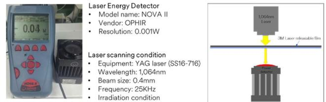
**Figure 10,** Laser energy blocking performance test, Measure transmittance of laser energy by using Laser energy detector (NOVA II)
