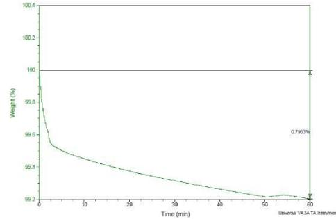
**Figure 4,** TGA Weight loss analysis of 3M Laser releasable temporary bonding film (multi-layered product): 0.793% @ 230 °C for 1hr, N2 Gas
