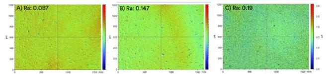
**Figure 8**, Surface roughness analysis of 3M laser releasable temporary bonding film (single layered product) by Bruker confocal, A) Ra value after glass lamination, B) Ra value after metal deposition (Cu), C) Ra value after thermal aging (@ 210 °C for 2hrs)
