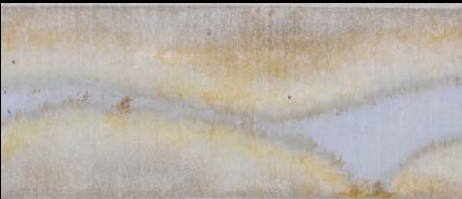
Other anodizing masking tapes are prone to leakage in harsh chromic acid baths
