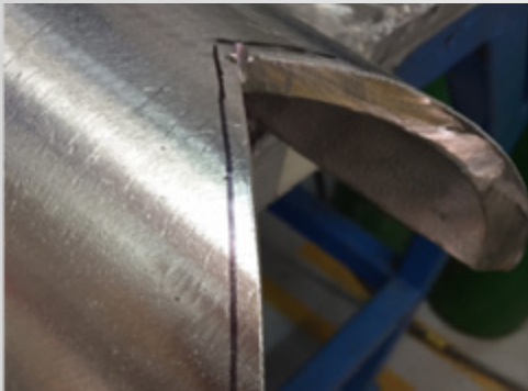
Weld prep marked
