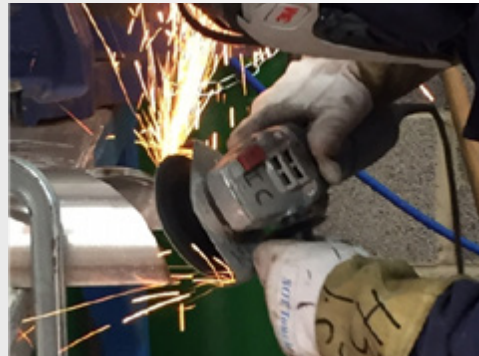
Weld prep – 3M™ 987C/787C 60+ Fibre Disc
