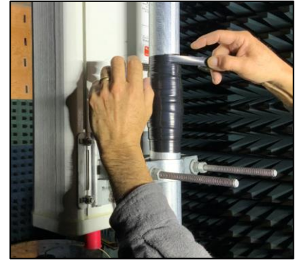
Minimize tension near end to prevent flagging
