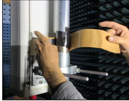
Wrap 3M tape 2122 with minimal stretch
