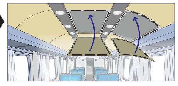
= Placement of 3M Dual Lock Strips
