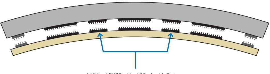
Additional 3M<sup>™</sup> Dual Lock<sup>™</sup> Reclosable Fastener strips can be applied to reduce vibration.
