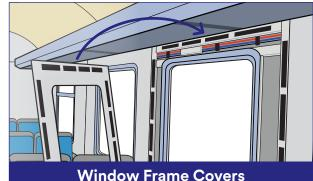
For easy access when replacement windows are needed. Can also cover wires, allowing access for service, if needed.
