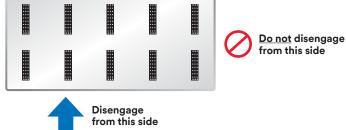
For panel bonding leave an opening corner or 4 opening corners To disengage start from any open corner, always working in one direction
