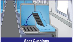
Fastened tightly to protect from theft or vandalism, yet maintenance friendly. Easily detachable for cleaning or refurbishment.
